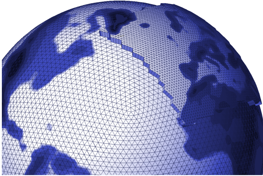
Figure 3.15.: Basic example of a multi-grid setup, consisting of a global ICON domain and a child domain over Europe with half grid spacing. This is similar to the deterministic forecast setup that is operationally used at DWD with a horizontal grid spacing of 13 km globally and 6.5 km in the child domain.
